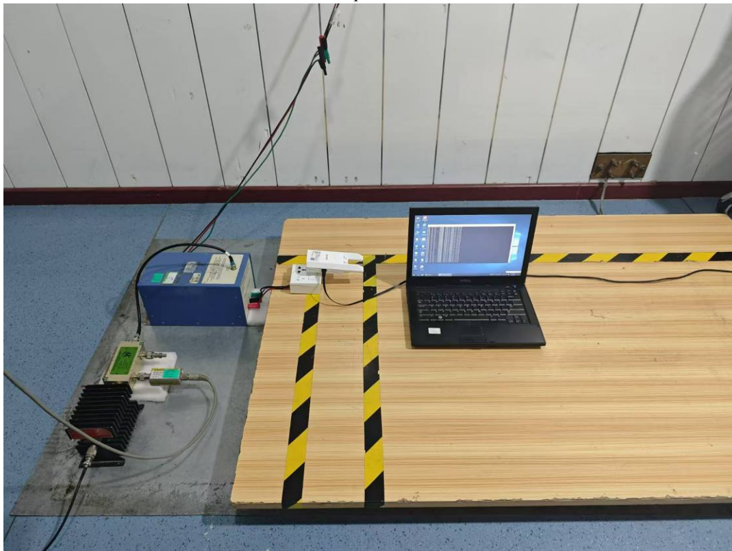
RJ45 Port Test Setup Photo View
