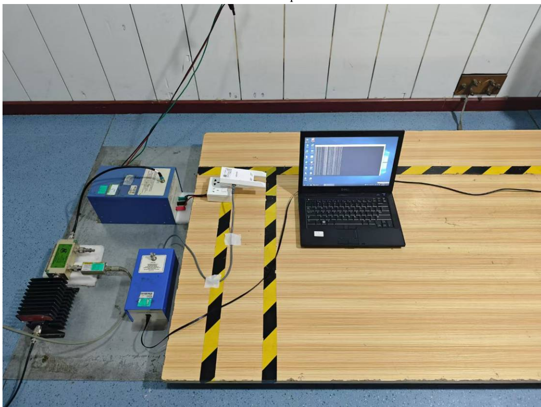
RJ45 Port Test Setup Photo View
